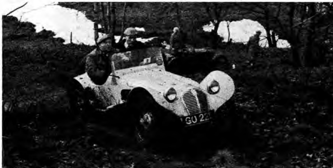
Gordon Gartside driving the trials car that had the first ever fibreglass body on a trial at Houden Clough.
