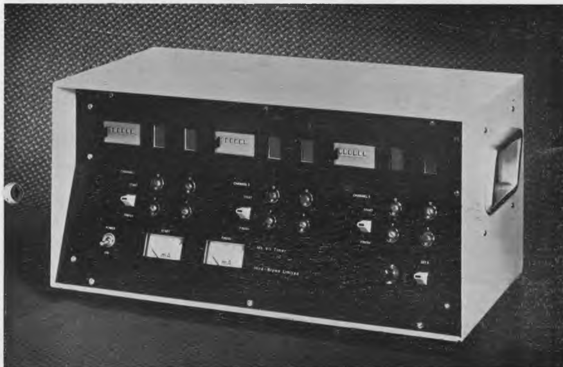
The heart of the Timing System is this electronic stopclock. The seconds and tenths are read out on the speedometer-like electro-mechanical counters whilst the hundredths and thousandths are projected in the small windows alongside each counter.
