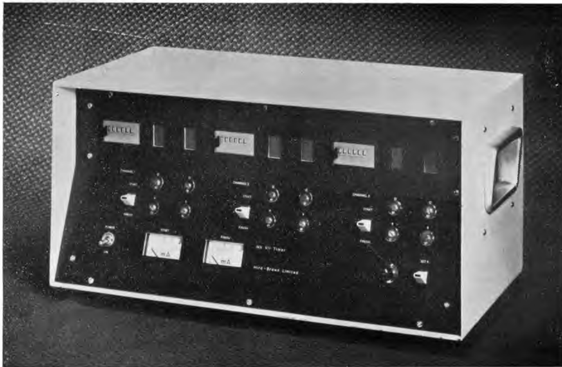
The heart of the Timing System is this electronic stopclock. The seconds and tenths are read out on the speedometer-like electro-mechanical counters whilst the hundredths and thousandths are projected in the small windows alongside each counter.
