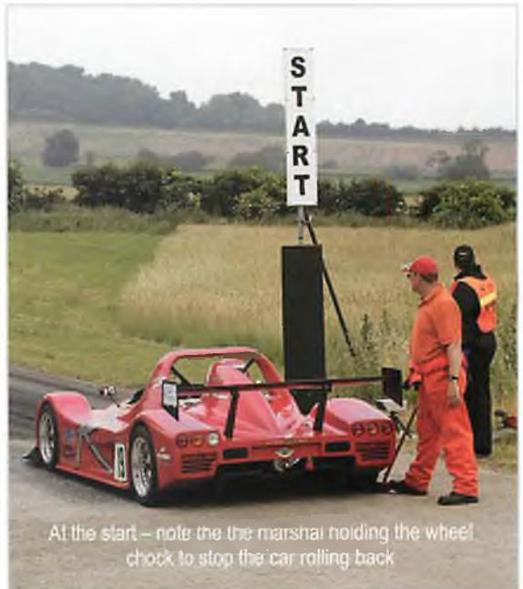
At the start – note the line marshal holding the wheel chock to stop the car rolling back
