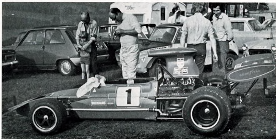
The Formula 1 DFV Ford engine tucks nicely into Sir Nick Williamson's Marlyn chassis.
